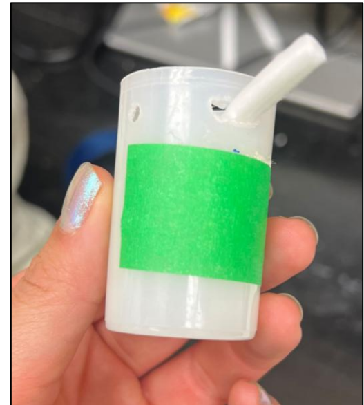
Hexanol filter (modified film can)
