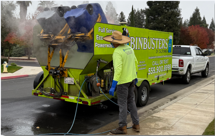
BinBusters of California utilizes a specially manufactured vehicle to sanitize bins and capture wastewater
