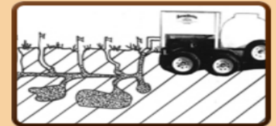
Diagram of how the Burrow Blocker effectively fills ground squirrel holes and burrows.
