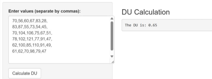
Figure 3. Screenshot from the online DU calculator reflecting measurements from our small 36 glass DU test.
