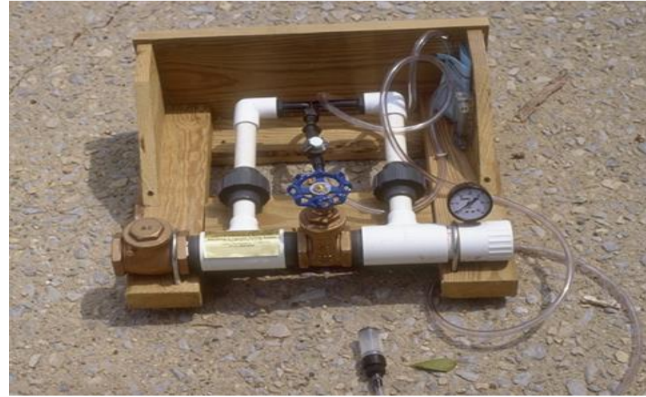
Venturi injector: Courtesy given by Dr. Timothy Coolong, UGA
