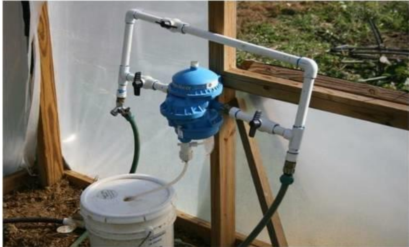
Greenhouse positive displacement injector: Courtesy given by Dr. Timothy Coolong, UGA
