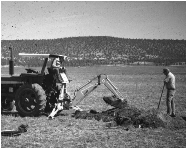
Figure 1.1. Use a backhoe to dig several evaluation pits in a potential field to determine the soil depth and to detect soil profile problems.
