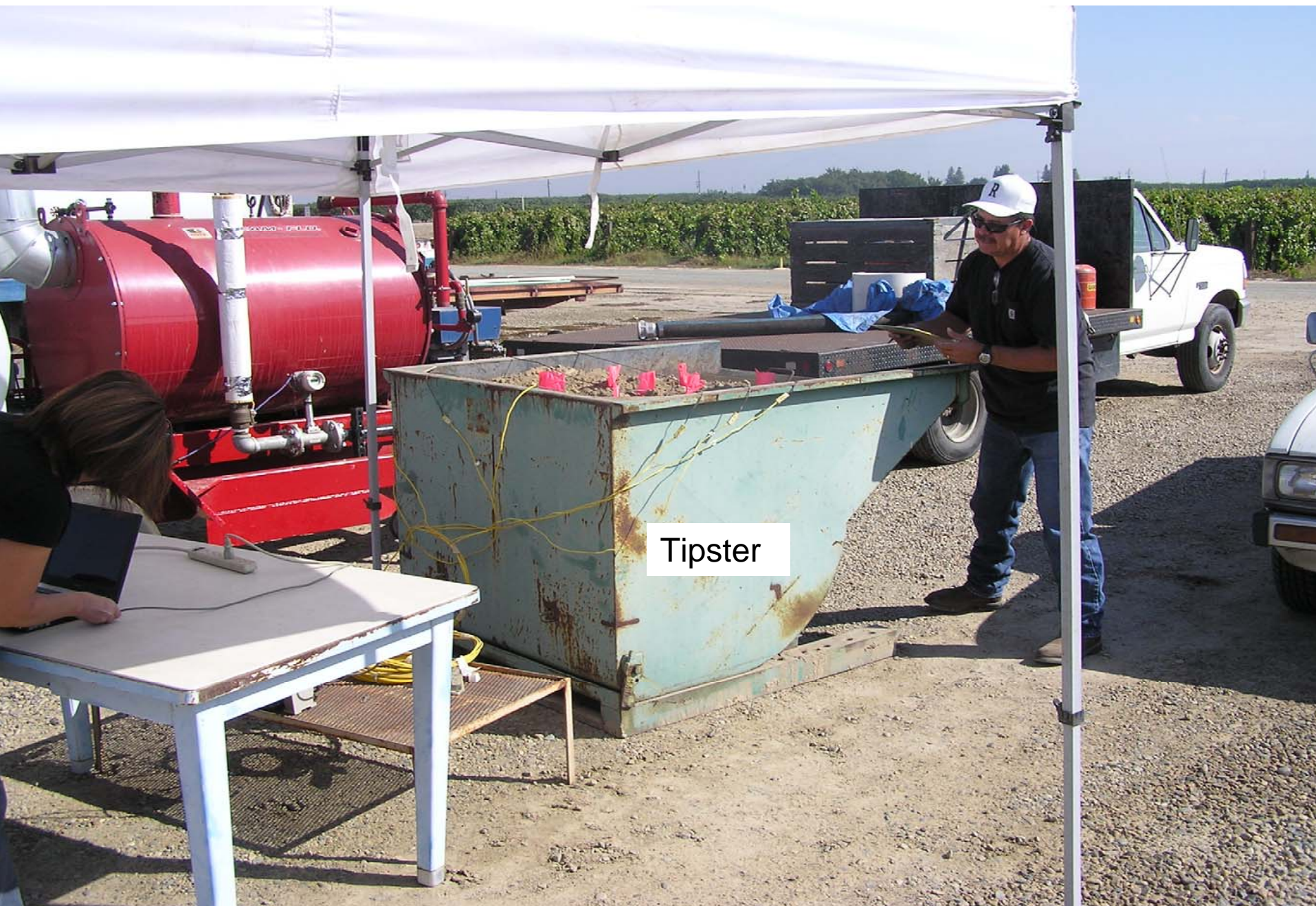
Tipster with thermocouples adjacent to our mobile steaming unit
