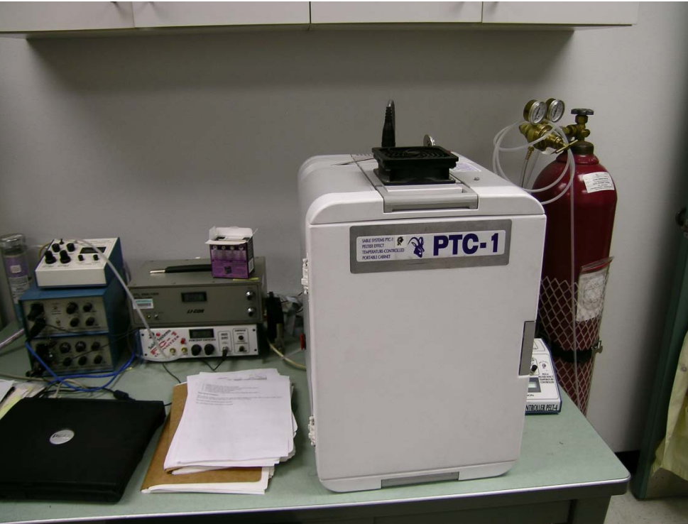
Respirometer measuring O_2 and CO_2 of individual bees
