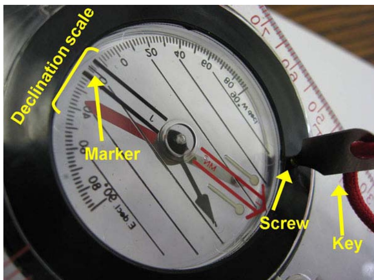
Figure 3-2: This compass has a special “key” that you use to turn a small screw on the bottom of the compass until the marker lines up with the appropriate value on the declination scale (read from the top side of the compass). Not all compasses do this the same way and some are not adjustable for declination—be sure to consult the instructions provided with your compass for details.
