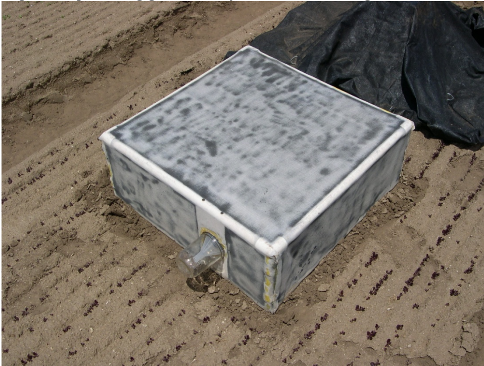
Figure 3. Emergence trap showing glass mason jar used for collecting the insects.
