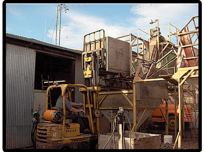
Picked nuts being dumped into hopper
