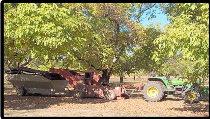
Tree shaker: grabs the tree trunk and shakes at a high frequency to knock the nuts to the ground.
